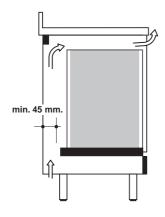
To provide adequate ventilation, there must be appropriate ventilation openings in the front bottom and the top part of the cabinet (an intake opening on the bottom of at least  $200 \text{ cm}^2$ , and an exhaust opening of at least  $60 \text{ cm}^2$ ).
